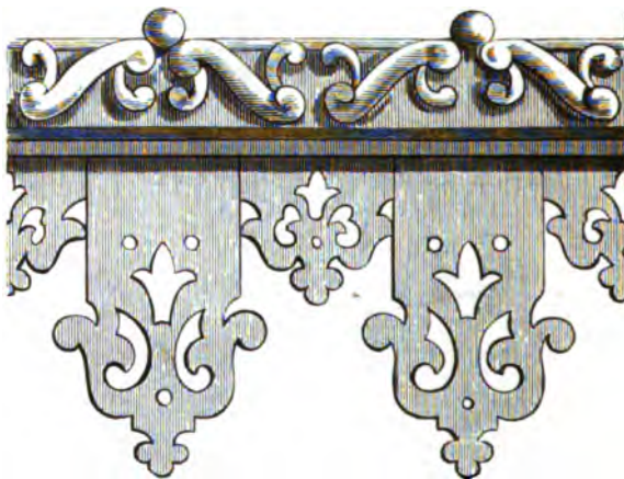
Elevation of zinc gutter, and cut woodwork.
