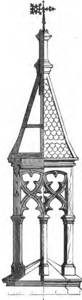
Half-elevation and section of bell-turret.
