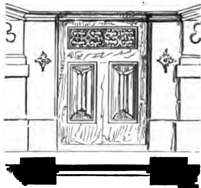
Plan and elevation of entrance garden-gate.
