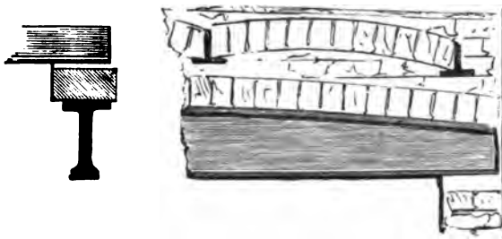
Section of kitchen roofing.
