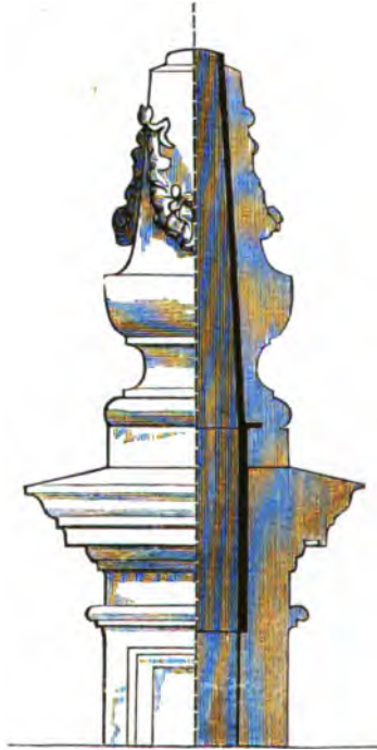
Chimney-pot elevation and section.
